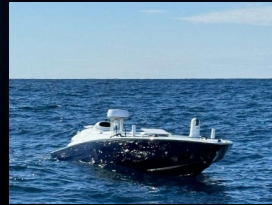
MINI-SEA RAPTOR 28 Autonomous and remotely controlled naval platform
